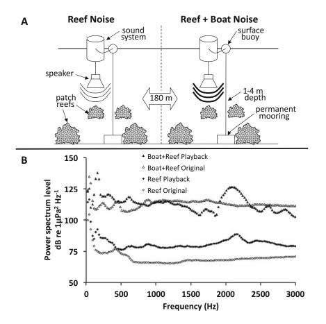
**Fig. 129.1** (a) Experimental study system showing configuration of reefs and underwater sound playback equipment. (b) Averaged power spectra (fast Fourier transform length 4096, 23.4 Hz bandwidth, Hamming window) for acoustic pressure levels in medleys of five original reef (*diamonds*) and reef+boat (*triangles*) recordings (*open symbols*) compared with recordings next to the patch reefs of the same recordings being played back through underwater speakers (*solid symbols*)
